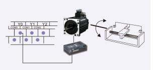
\*Note: when using high-speed pulse output function, the PLC can output 100KHz  $\sim$  200KHz pulse, but can not guarantee the normal operation of all servos.
